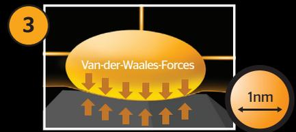
Superior adhesion to the road surface created by molecular forces - based on the "Van-der-Waals-Forces" - which bonds the polymers to the road surface on a nanometre level.
